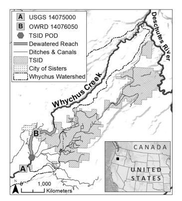
FIGURE 1. Whychus Creek watershed, showing Whychus Creek and relevant features circa 1995 (i.e., before transactions), including streamflow-gaging stations (A and B); TSID POD, water distribution network, and irrigated lands; and the dewatered reach below the TSID diversion. Note that a large portion of the irrigated land lies outside the watershed. USGS, United States Geological Survey; OWRD, Oregon Water Resources Department; TSID POD, Three Sisters Irrigation District's point of diversion.
