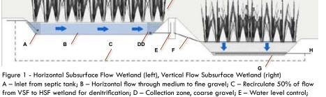
F – Intermittent dosing of VSF; G – Water drains vertically through gravel to bottom drain; H – Outflow to free water wetland; I - Dense planting. For the plan view of the HSF and the VSF wetland see Figure 2.
