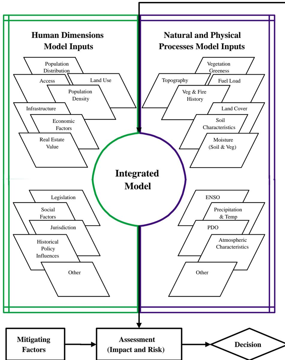
**Figure 2.** Schematic diagram of the factors used in the integrated model, including socioeconomic factors, as well as land use and climate factors.
