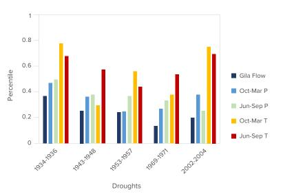
Multi-year droughts in the gage record for the Gila River, with water year streamflow, cool and monsoon precipitation and temperatures averaged for the years in each period of drought. Values are in percentile and color-code to correspond to the different variables.
