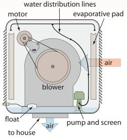
Swamp coolers typically consist of a box with vented sides. A fan draws ambient air through vents and through pads that are kept moist by a water supply, pump, and distribution lines. The cooled, moist air is then delivered to the building via a vent in the roof or wall.
